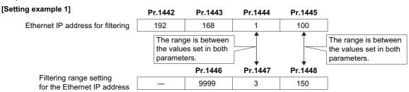
In this case, the IP address range in which Ethernet communication is permitted is "192.168.x (1 to 3).xxx (100 to 150)".
